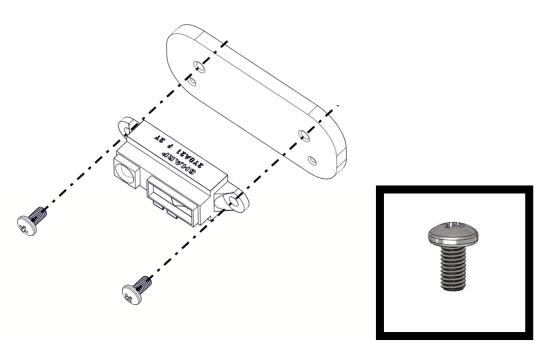
9. Insert the distance sensor plate into the slot in the front of the robot using two M2 x 6mm screws (am-1553). No nuts are used, these screws thread into the plastic.
