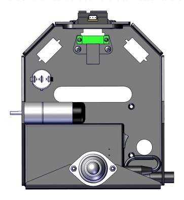
15. Install the motors using four M2 x 6mm Pan Head Screws (am-1553).
