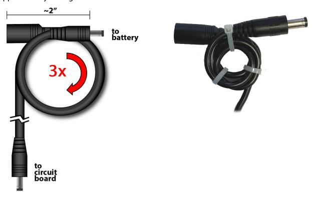
5. Plug the shorter male end of the Battery Cable to the Battery and slide the Battery into the rear right corner of the chassis. The lights on the battery should face out and the switch should be located on the left.
