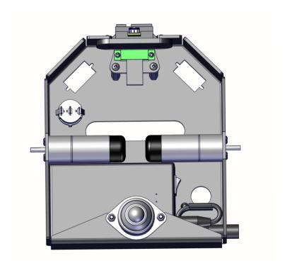
17. Press one Wheel (am-4354b) onto each motor shaft. Ensure the D-shaped profile of the shaft aligns with the D-shaped profile of the wheel bore.
