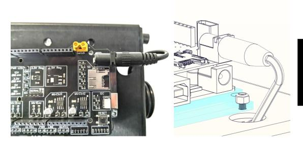
Note: Be sure to plug into the top Skitter Board and *not* the Arduino.
