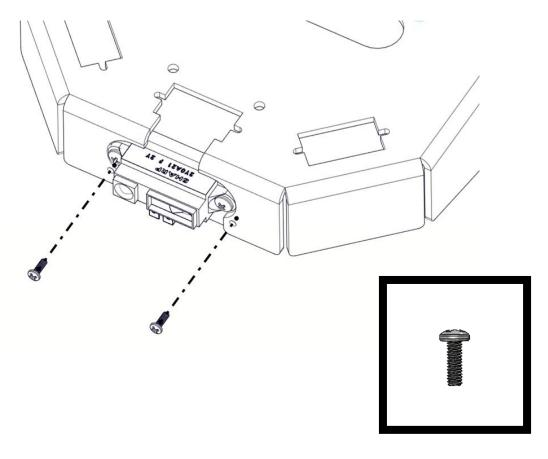
10. Mount Standoffs (am-1729) to underside with two M3 x 6mm Pan Head Screws (am-1556) in the holes as shown.
