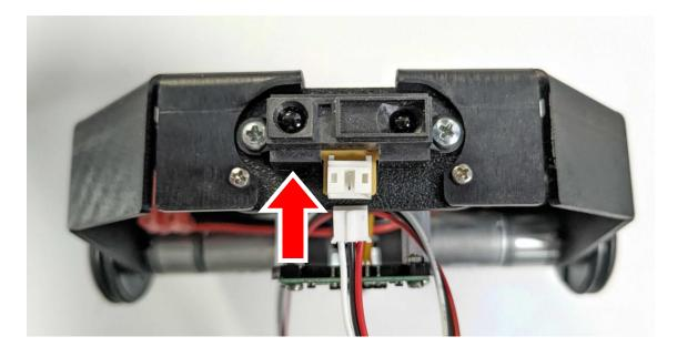
24. Plug in the distance sensor cable (am-5479) into the LIDAR connectors on the Circuit Board.
