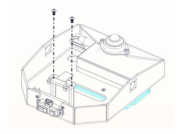
14. Align the Gearmotor (am-4513) with the hole in the side of the frame. Note: To ensure the wires are cleanly routed, rotate the Gearmotor to align with mounting holes so that the wires route under the motor but still allow for a small amount of slack for the connection to the Circuit Board.
