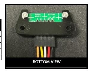
13. Secure the line follower sensor to the standoffs with two M3 x 6mm Pan Head Screws (am-1556). The sensors on the circuit board should be facing outwards and away from the frame.
