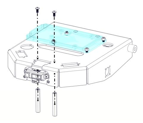
11. Attach the Line Follower Sensor (am-4857) to the Line Follower Sensor Bracket using M2 x 6mm Screws (am-1553) and M2 Nuts (am-1554).
