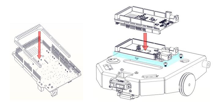
22. Feed the motor cables neatly through the slot in and plug into the Circuit Board as shown.
