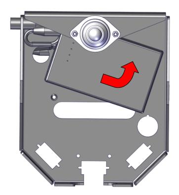
7. Snap in the On/Off Switch (am-3797\_switch) into the mounting hole in the frame. Ensure the locating key on the switch is aligned with the notch in the frame.
